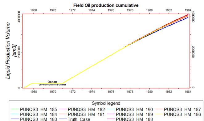
**Data Match.** Production data generated from model realizations based on an optimizer solution.
